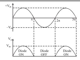
⇒During +ve half cycle of supply voltage diode on and during –ve half it is off.
